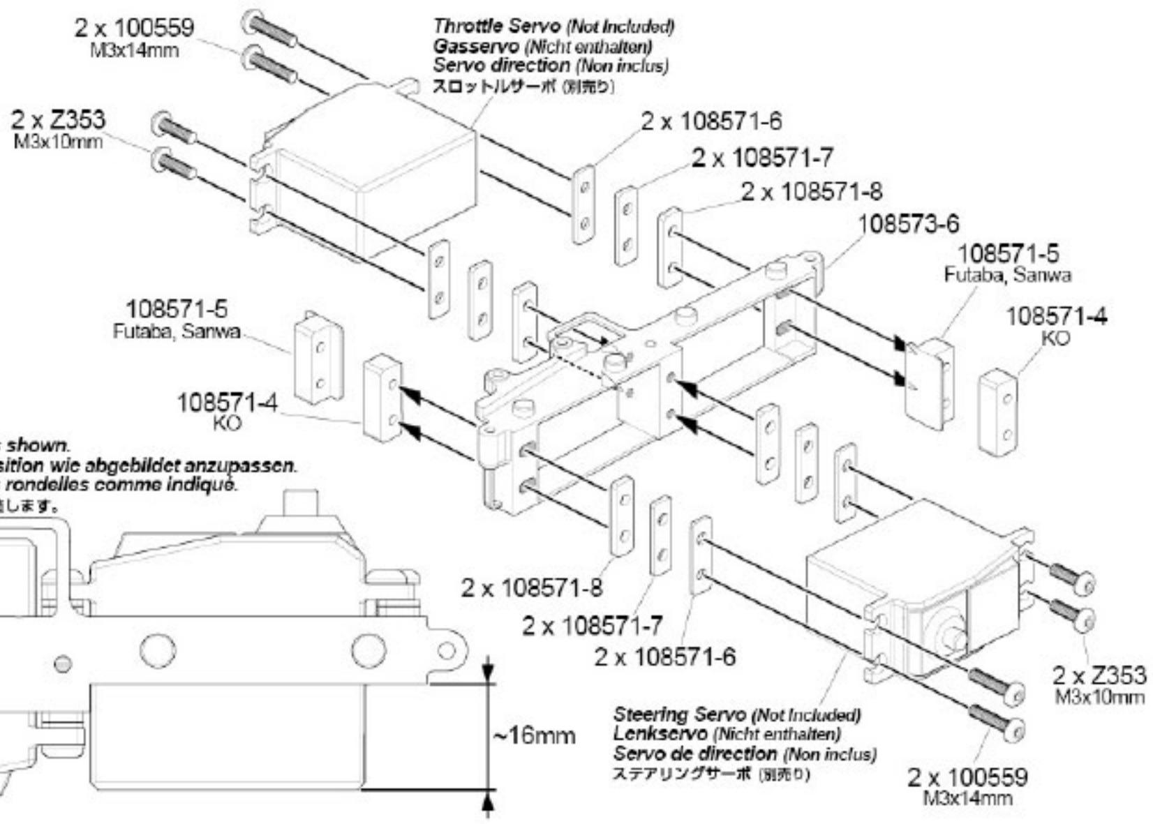
Adjust servo position using spacers as shown.
