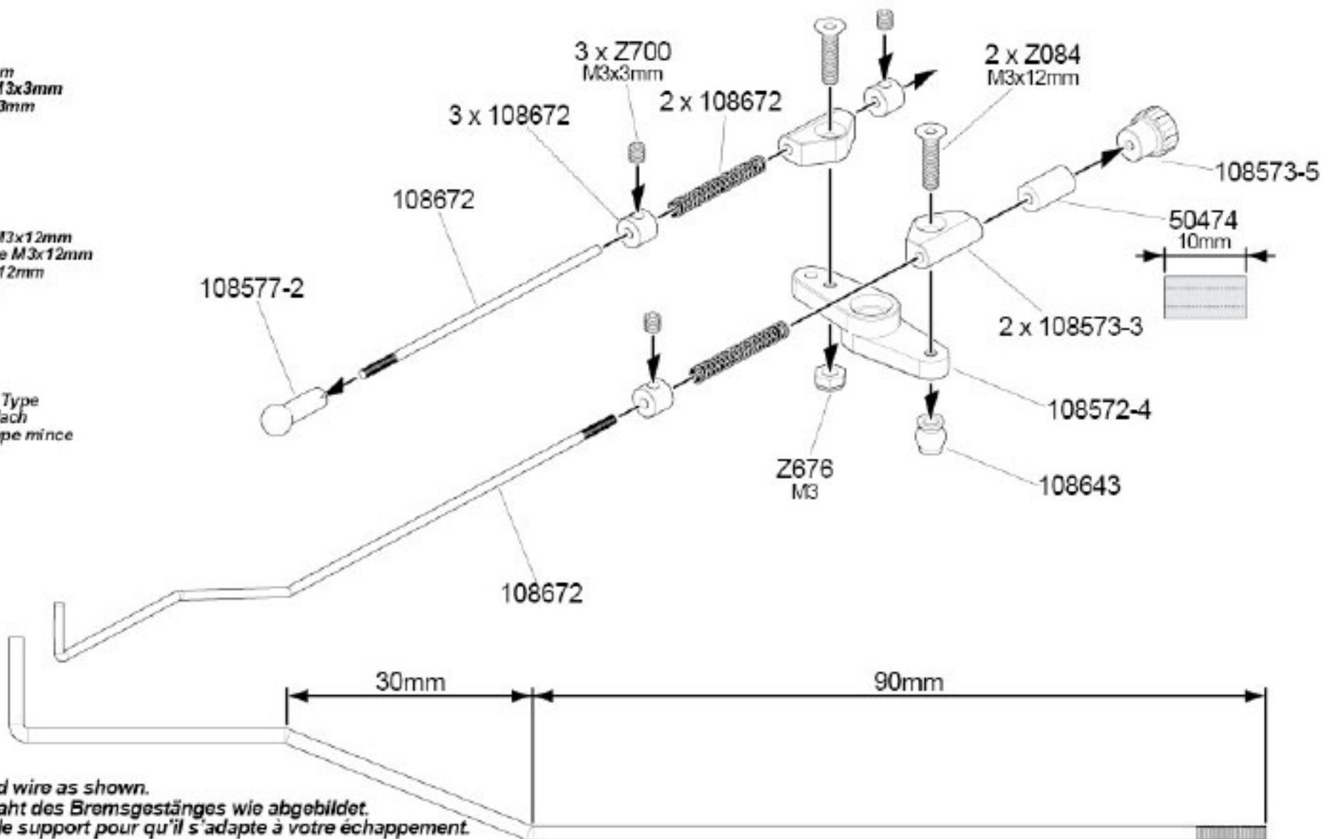
Bend the brake rod wire as shown.
